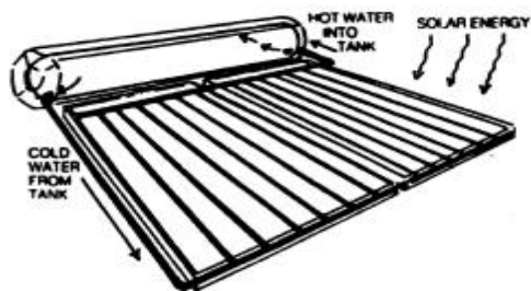
How solar water heating works A typical close-coupled thermosiphon solar water heater
